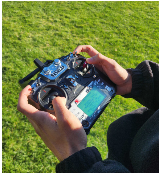
Figure 20: Manual control override with controller
