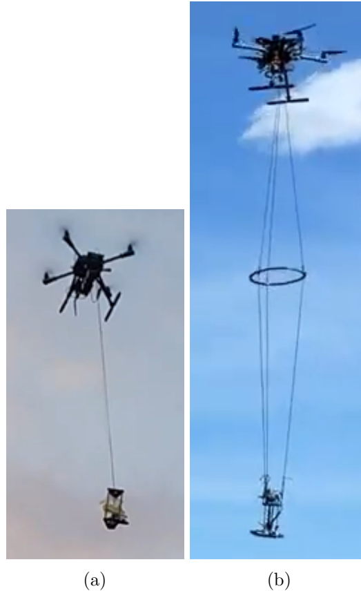
Figure 27: (a) Single-point mounting (b) Multi-point mounting with bridle ring
