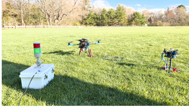
Figure 19: Audio-visual safety alert at the system Ground Station using a safety lighthouse
